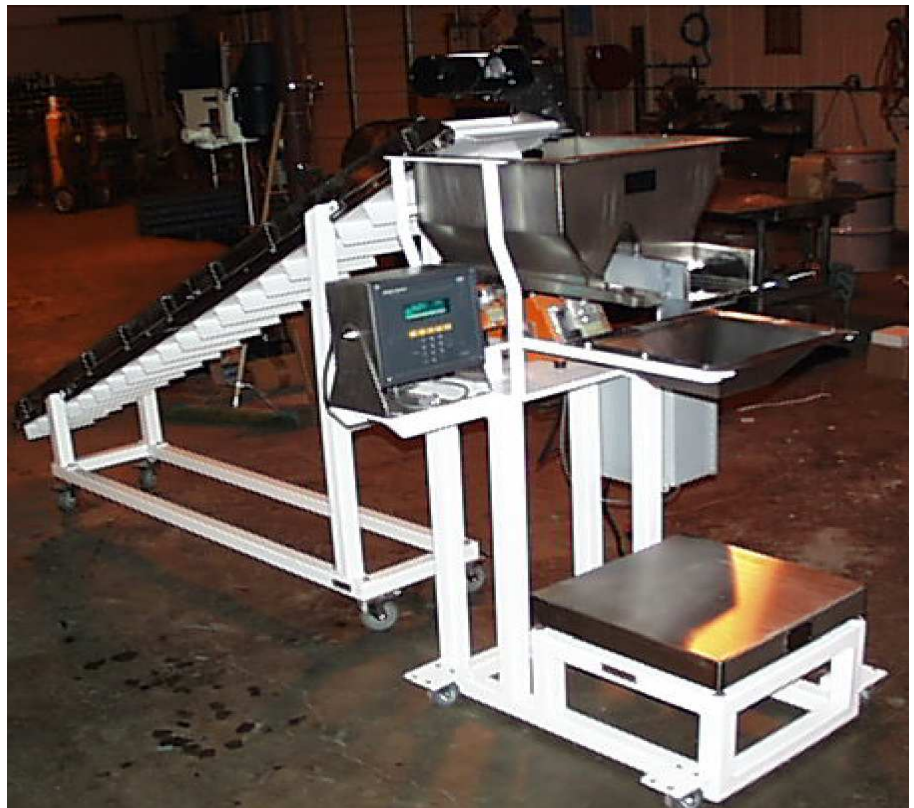
PS-10 Semi-automatic bulk packaging system for a cinnamon sugar topping mix with the portability option
