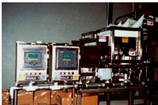
PS-20-Dual Auto Indexing bulk packaging system for frozen bakery products (bagels & bread sticks)
